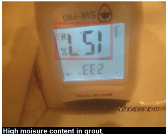
High moisture content in grout.
