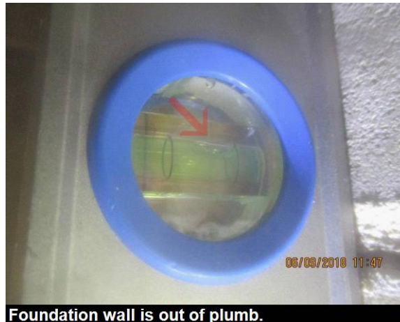
Foundation wall is out of plumb.
