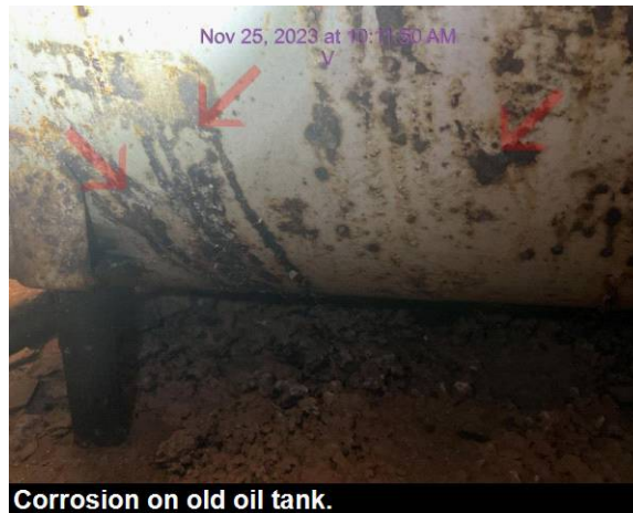
Corrosion on old oil tank.
